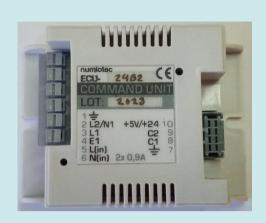
numioECU family is a device specially designed for lights electronic control, in hospital bed head units. The system allows commuting one or two lights by means of a double control and/or two conventional push buttons
